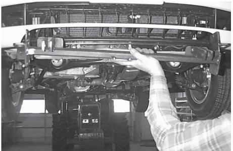
3. Install cross member with three 3/8" x 1-1/4" hex bolts, lockwashers and hex nuts on each side.
